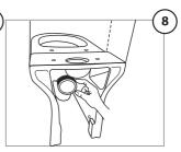
· Apply suitable lubricant around waste outlet before connecting to the bend.
